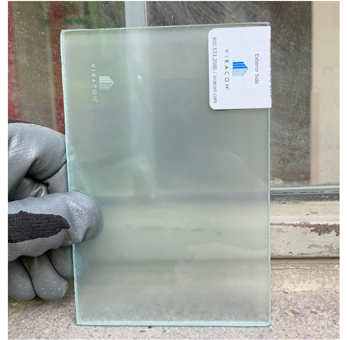
Sample of proposed ceramic frit for canopy glass. Note that this photo only represents the opacity of the ceramic frit. Color rendition of the glass will be similar to G-1.
