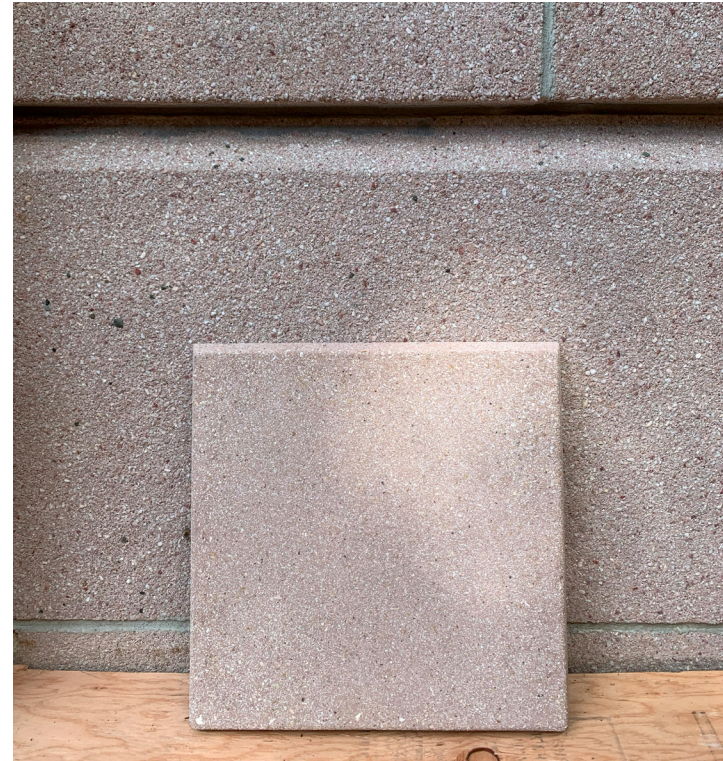
Proposed cast stone sample with existing historic cast stone. Overall colors will match, but new stone will have a slightly finer, more smooth aggregate.
