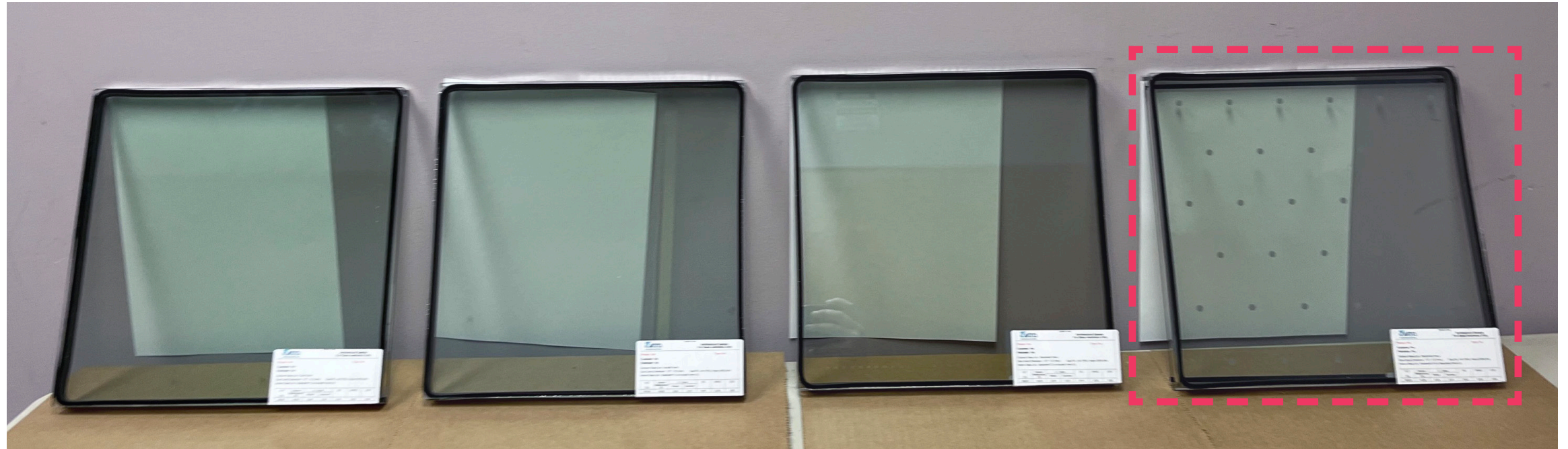
Considered glazing assemblies with most amount of iron content on the left and least amount of iron content (Starphire/Starphire- proposed highlighted with red dash outline) on the right
