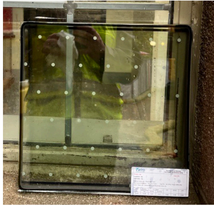
Bird strike deterrent ceramic frit pattern. 1/4" diameter dots, 2" x 2" staggered, approximately 1% coverage. Note that the bird strike deterrant pattern has been applied to surface #4 and this photo is meant to illustrate pattern & color only
