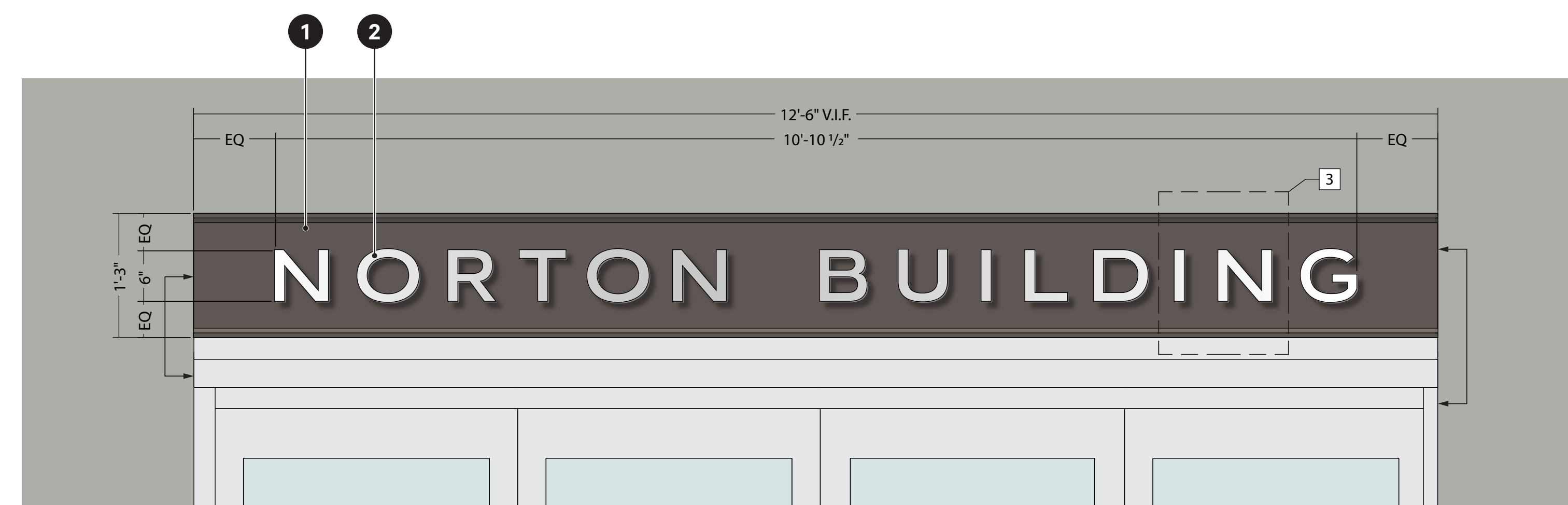
1 ID2: Secondary Building ID—Elevation Scale: 1" = 1'-0"
